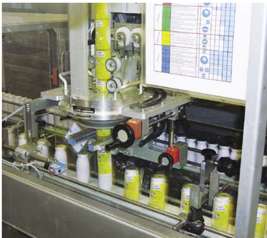
One of Dannon's goals is to ensure that bottles of DanActive dairy drink arrive in stores on time. Its camera system tracks machine jams and other maladies on-the-fly.
