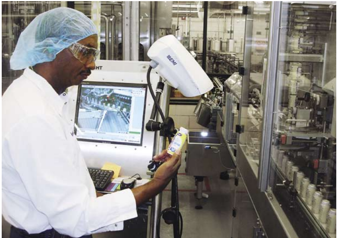
Jerry Shoemaker, plant technical manager, operates the camera-based video-inspection system in Minster, OH.
