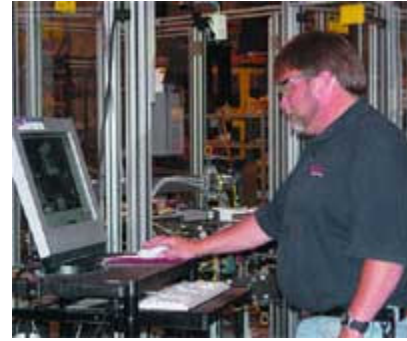
Winger calibrates the timing of an air cylinder on the KD case packer through the video monitor workstation.
